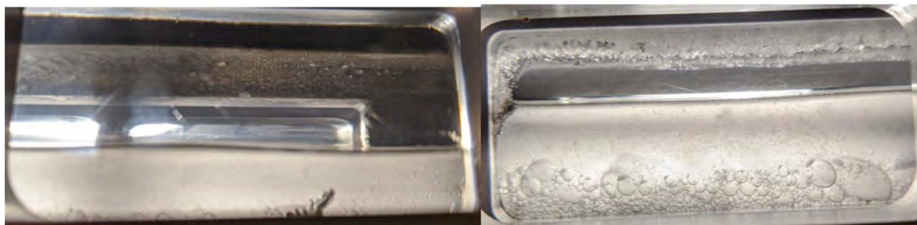
Figure 1—Condensation of water droplets in gas phase (a, left) that resulted in hydrate film upon nucleation (b, right).
